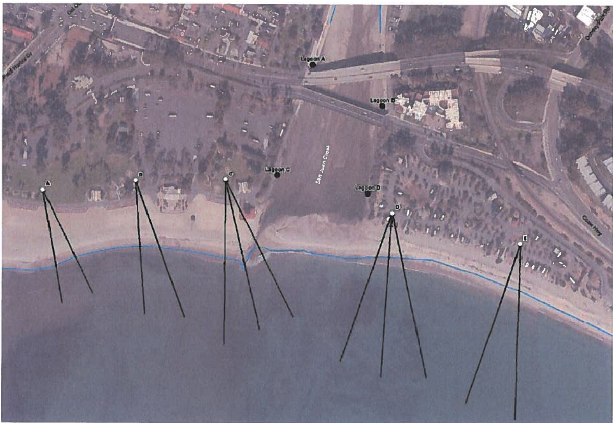
Figure 1. Subsurface slant well layout along Doheny Beach (white circles, A-E) adjacent to San Juan Creek Lagoon (black lines show alignment only) including evaluation sites (black circles, A-D), which will monitor changes to the shallow aquifer under the lagoon (source: Draft Environmental Impact Report (DEIR), Figure 8 in Appendix 10.10.1).
